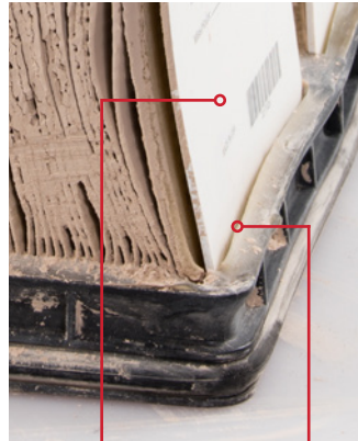
Structural Bowing, resulting in glue-bead separation
