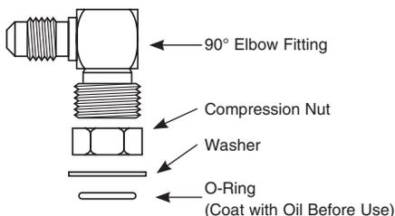
**Note:** Mount Model Before Installing Fittings. O-Ring Seal Fittings Require Care in Installation. **DO NOT OVERTIGHTEN.** See Instructions Below.
